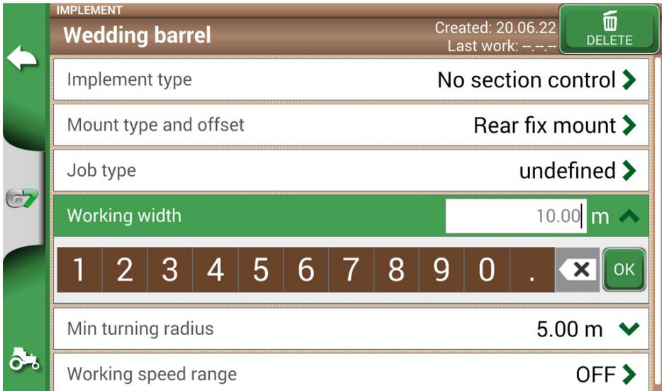
Figure 2.1.6.j - Tractor minimum turning radius setting
