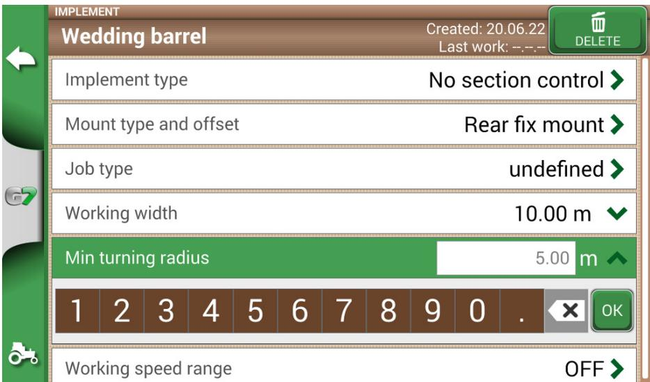
Figure 2.1.6.h - Working width setting
