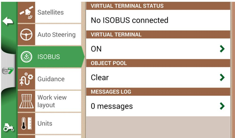
Figure 2.4.4.a - ISOBUS active, not connected
