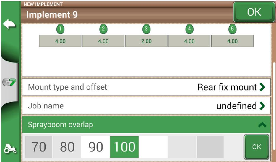
Figure 4.9.k - Spray boom overlap configuration
