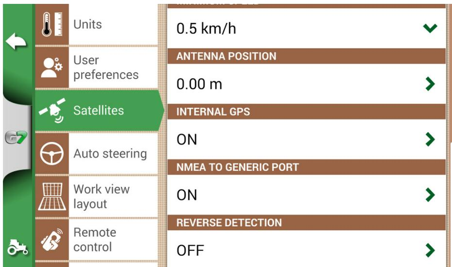
Figure 6.6 - Virtual GPS output on the 'Generic' port
