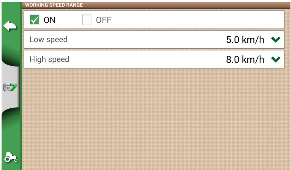
Figure 2.1.6.k - Activation and definition of working speeds
