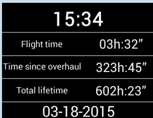
Clock Page: flight time, time since the last service overhaul, life time of the engine.
