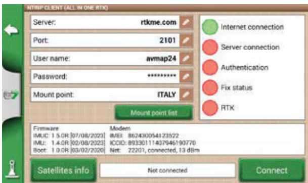
Figure 6.1.2.b - NTRIP Client configuration
