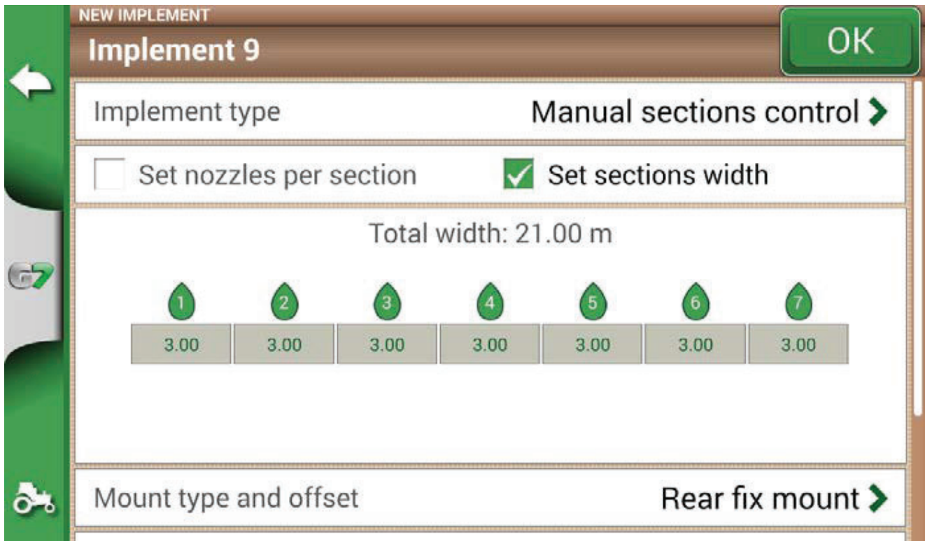
Figure 4.10.f - Sections configuration: section width
