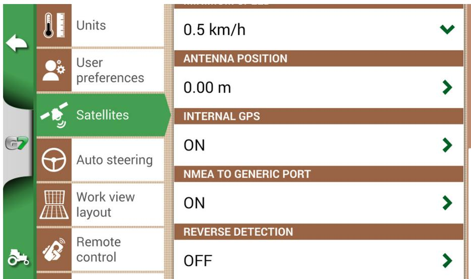
Figure 6.6 - Virtual GPS output on the ‘Generic’ port
