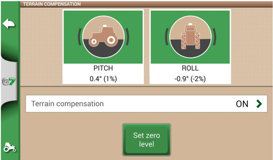
Figure 2.4.1.c - Terrain Compensation Activation, Pitch / Roll Display
