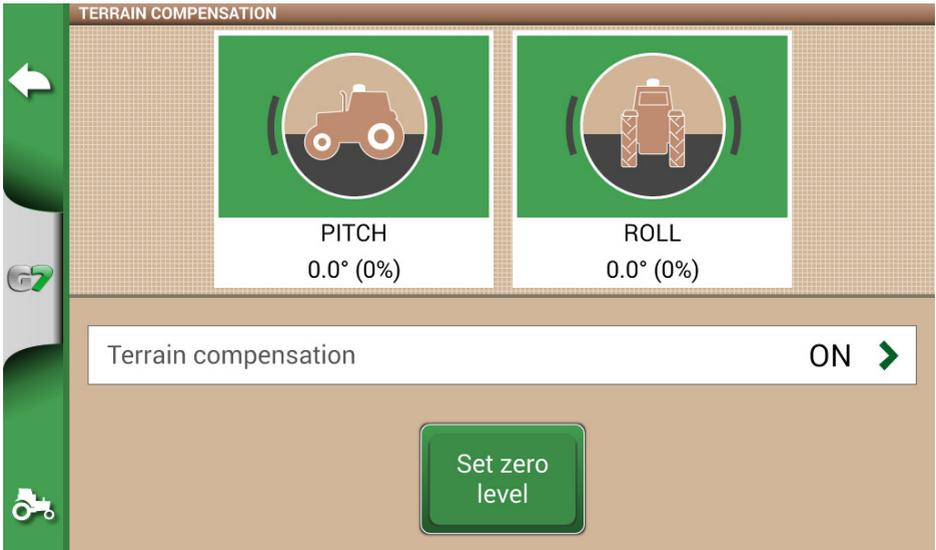
Figure 2.4.1.d - Zero calibration of the ground compensation
