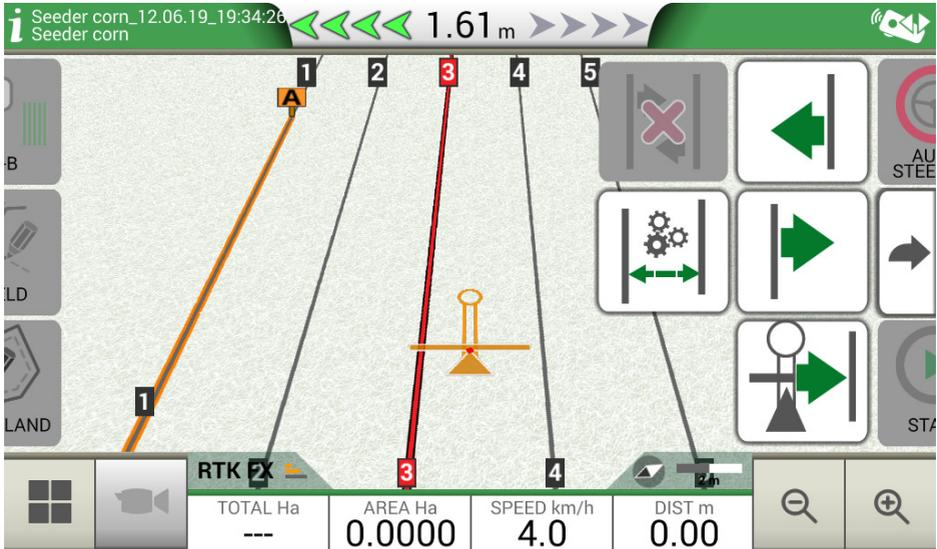
Figure 3.2.7 - Work page, A-B lines movement.
