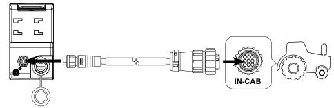
**ATTENTION:** The In-cab cable is not waterproof. Do not use outside the tractor cab.
