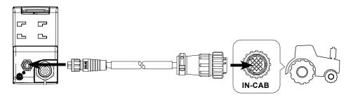
ATTENTION: The In-cab cable is not waterproof. Do not use outside the tractor cab.
