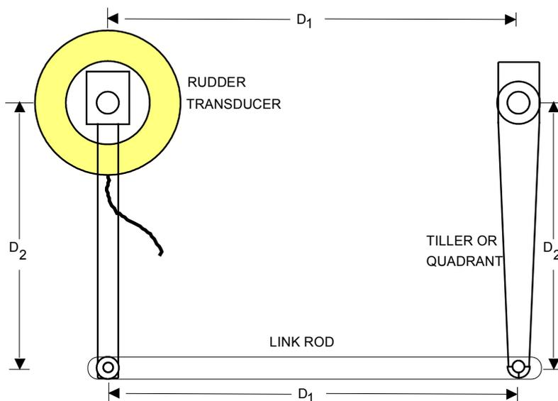
Figure 3.6 S81.03 Rudder Transducer Linkage
