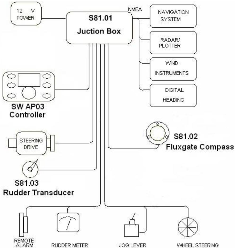
Figure 1.5 Autopilot system using the S81.01 Junction Box.
