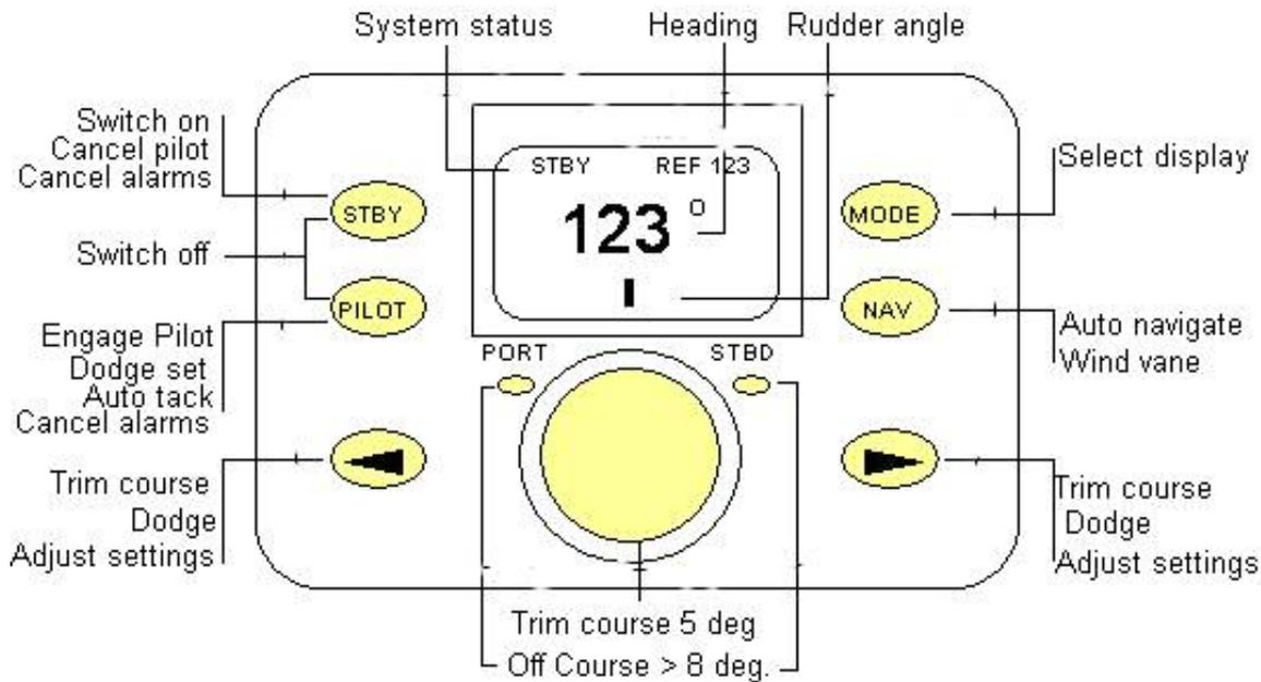
Figure 2.1 The AP03 Controller panel.
