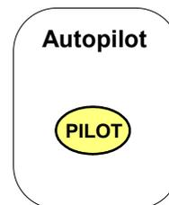
With the system in STANDBY, steer the vessel to the desired heading and press PILOT. The autopilot will now lock onto that heading and maintain it. The position of the rudder when the PILOT key was pressed is stored in memory as the effective helm centre. The display will show 'PILOT' in the top left corner.
