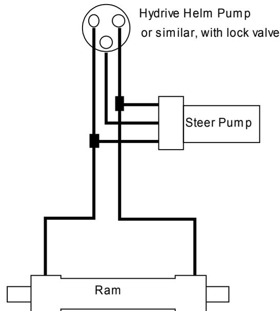
Figure 3.13 Connection to a typical two-line system
