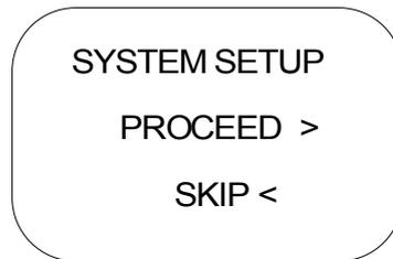
There are two choices. If you wish to examine some of the features without carrying out the setup, select SKIP by pressing the left arrow. This will bypass the setup and let you scroll through the displays, but there will be no response to the PILOT key. The system will return to SYSTEM SETUP the next time it is turned on.
