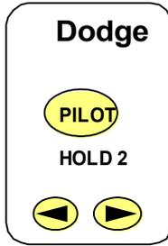
The dodge function is used to make a quick course change to avoid an obstacle. Hold the PILOT key down for two seconds, a beep will sound and the dodge message appears in the top left hand side of the display. Release the key and press the left or right arrow keys to run the helm out. When the arrow key is released the helm holds its current position. To return to the original course, press PILOT.
