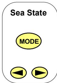
Press the MODE key once. The display shows the current control mode setting.
