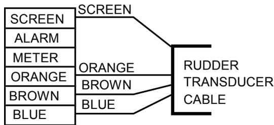
Figure 3.7. Rudder transducer connections.
