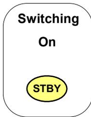
Press the STANDBY key. The system does a self-test for a few seconds and displays the version of software fitted to your autopilot. When the self-test is complete the normal STANDBY display appears and shows the current heading of the vessel.
