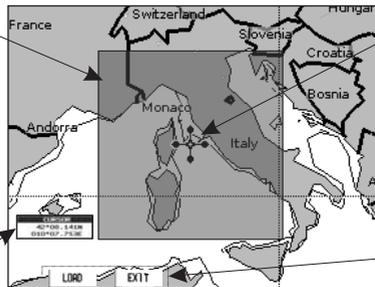
Cursor is locked to the gray area. Moving the cursor also moves the gray area allowing locating it over the area where the user wants to download the Meteo forecast.
