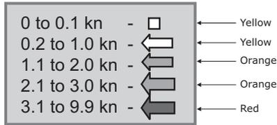
When the chart plotter receives a valid position fix, the Tide icons are shown on the charts on the basis of the current date and time: the screen displays and changes arrows as date/time changes.
