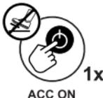
2. The ignition is switched on without the brake pedal being pressed
